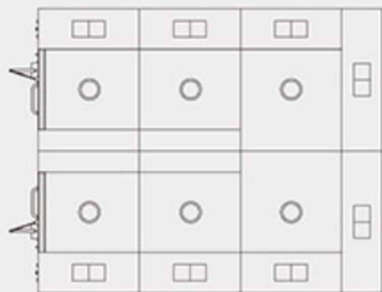
U-shaped air shower tunnel
